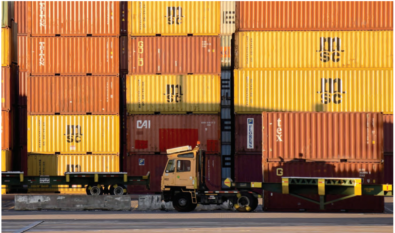
Four manufacturers already offer electric versions of yard trucks, which move cargo containers within port, railyard, and warehouse complexes.
